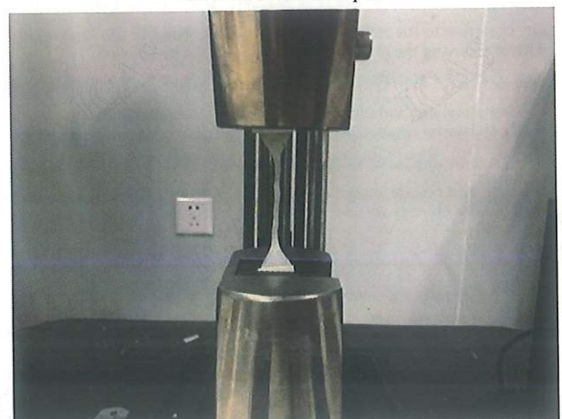
During Breaking force before aging test
